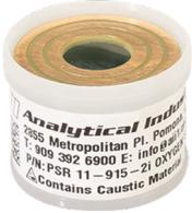
Advanced galvanic type % oxygen sensors with excellent stability and accuracy under stringent applications. All % oxygen sensors are subjected to the most extensive stability test, output in air, 30" of water column pressure test and stability at 100% oxygen.
