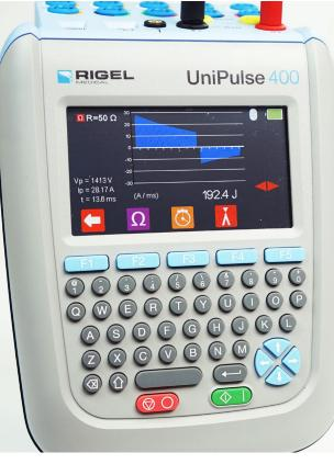
The new **UniPulse** 400 is designed to comprehensively test all defibrillators accurately and efficiently. The large vibrant color screen will display both test results and waveforms in amazing detail. The dedicated fast keys and simple to use operating system enables biomedical/clinical engineers to select the relevant test function in seconds.
